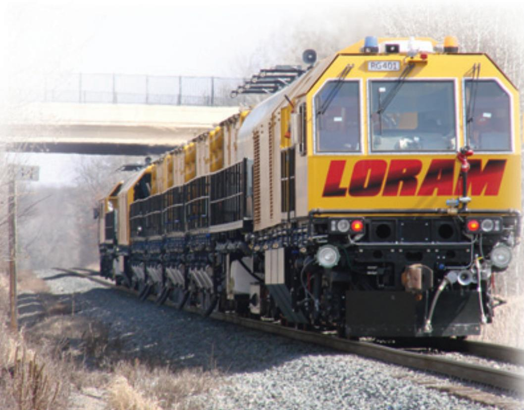
**Loram's new RG400 series high-production grinders offer higher stone counts and shorter machine lengths.**
