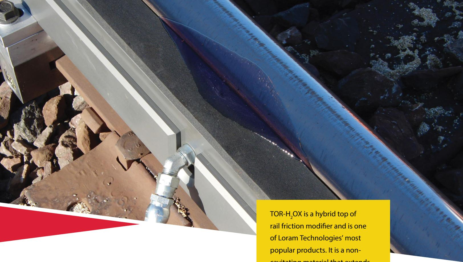
TOR-H<sub>2</sub>OX is a hybrid top of rail friction modifier and is one of Loram Technologies' most popular products. It is a non-cavitating material that extends the life of wheels and rail.
