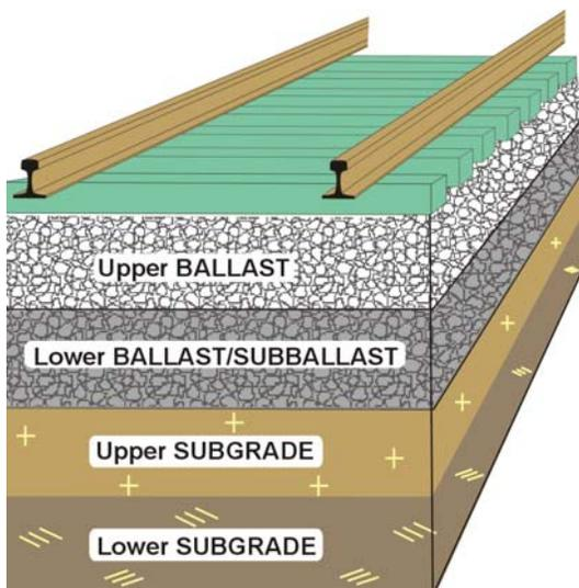
Figure 1: Idealized track substructure.
