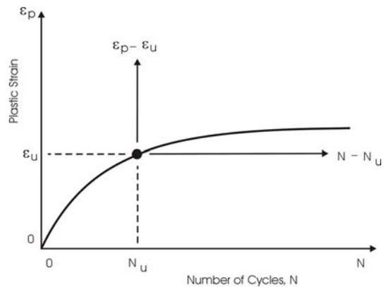
Figure 3: Stress-strain characteristic of soil subjected to repeated loading.
