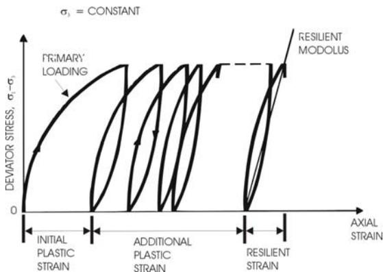
Figure 2: Cumulative Strain and Stiffness of Materials Under Repeated Loading
