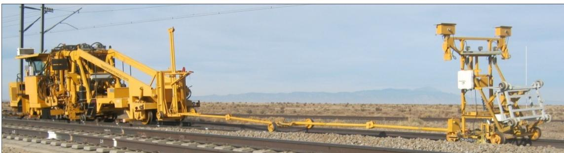
**Figure 3. Track Surfacing and Alignment Machine**
