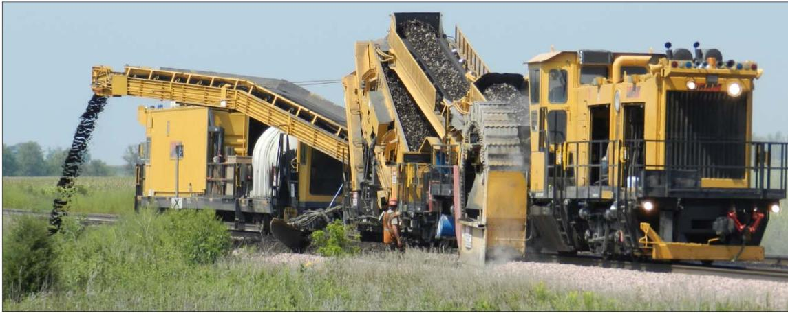
Figure 23. Loram Ballast Shoulder Cleaning Consist
