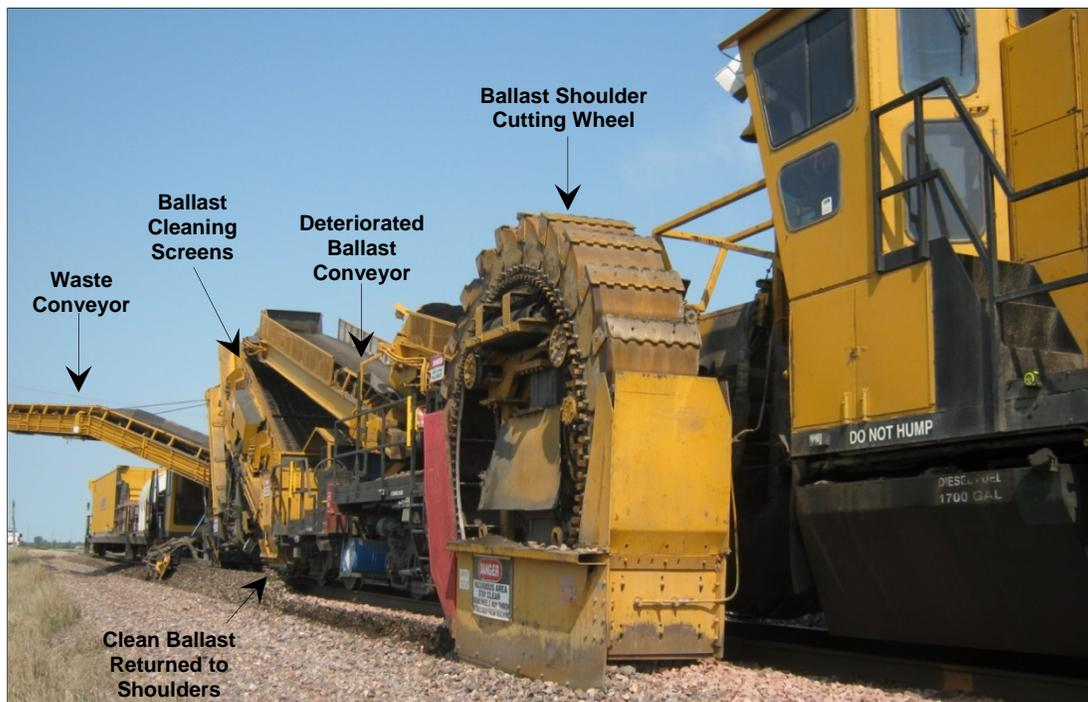
Figure 24. Details of Loram Ballast Shoulder Cleaning Operation
