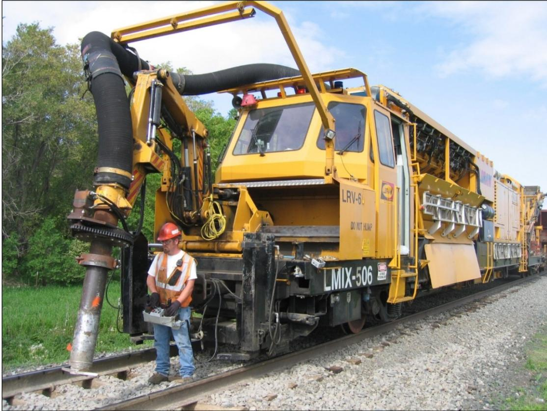
Figure 12. Loram RAILVAC™ Ballast Vacuum Machine<sup>6</sup>
