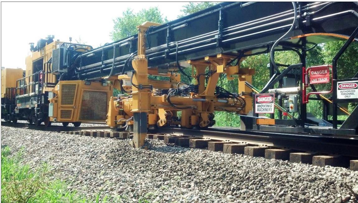
**Figure 10. Loram Track Lifting Machine<sup>5</sup>**
