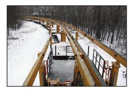
Capable of loading and unloading in curves up to 12 degrees.
