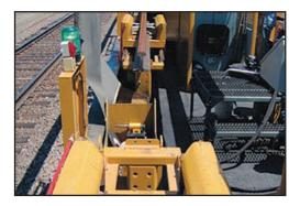
Rail cutting and joining is centralized on the work unit.
