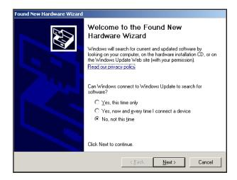
Allow the wizard to install the software automatically. Windows should search the SENSR CD for the appropriate drivers. If the wizard cannot find the correct software, you can install from a specific location. The drivers are located on the SENSR CD in the Drivers\Sensr GP Series Device Drivers Vx.x.x
