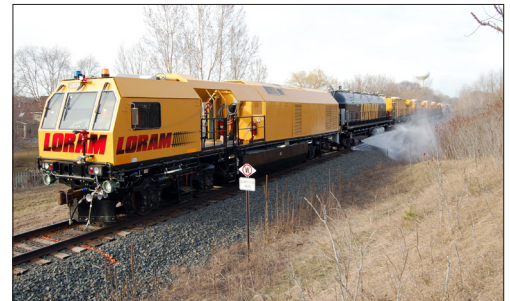
Modular design allows specification of 60–120 grind stones
