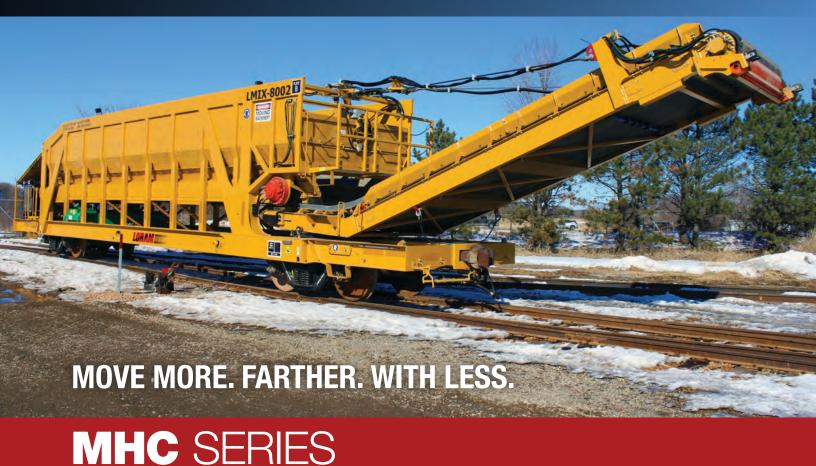
**Loram's MHC Series Material Handling Cars** are ideal for any project involving transferring and offloading of new ballast, or excavated roadbed materials such as ballast and spoils. Featuring a powerful, integrated transfer conveyor based on proven Loram components, the MHC Series provides a continuous, high-throughput flow of material for maximum productivity.
