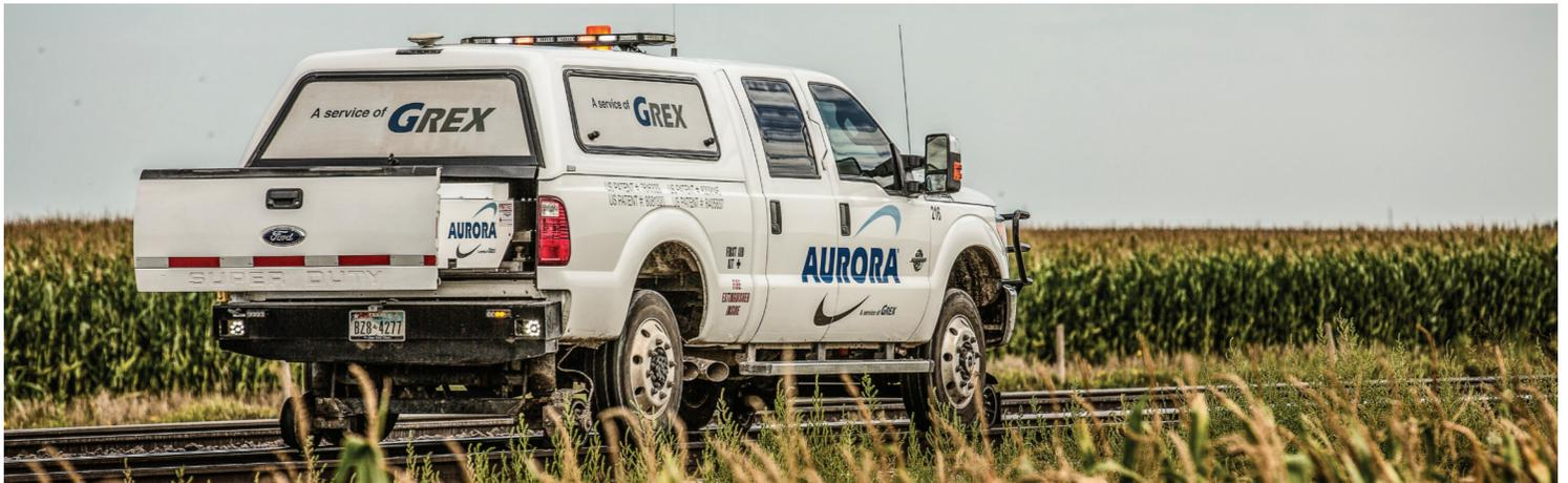
The Iowa Interstate Railroad used the GREX Aurora<sup>®</sup> tie inspection system to evaluate the tie condition of more than 120 miles of track.
