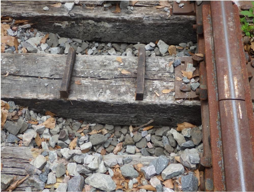
Figure 8: Sleeper surface before destructive examination. The void in the X-Ray image is between the two cross-member timber blocks.
