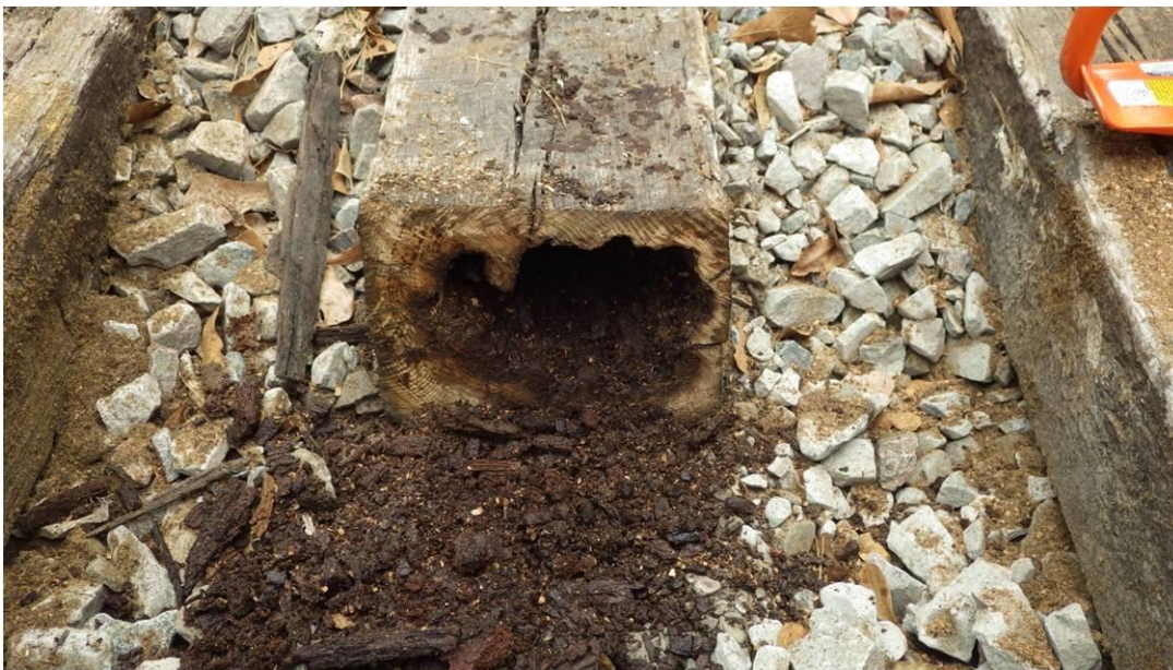
Figure 9: Sleeper surface and subsurface after destructive examination. The void is readily apparent.
