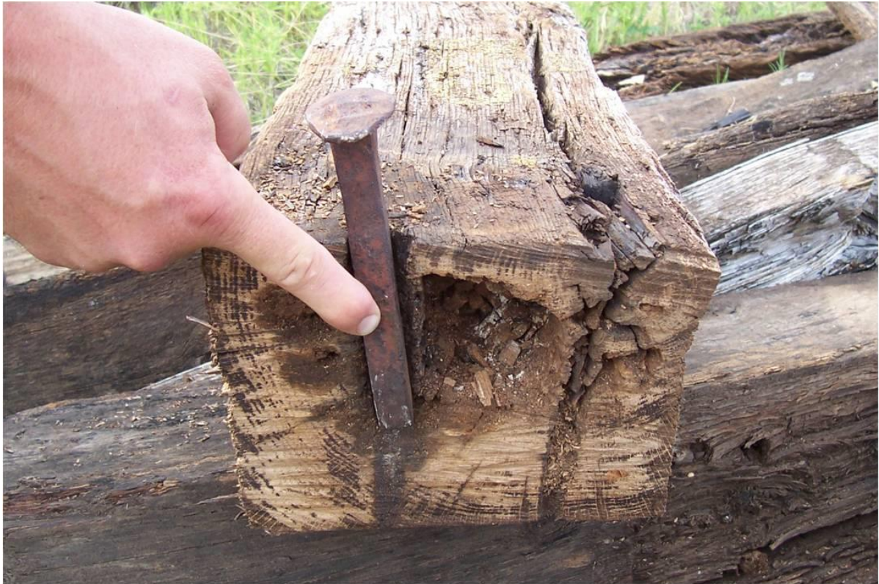
Figure 2: A Subsurface Defect is shown in proximity to a spike hole
