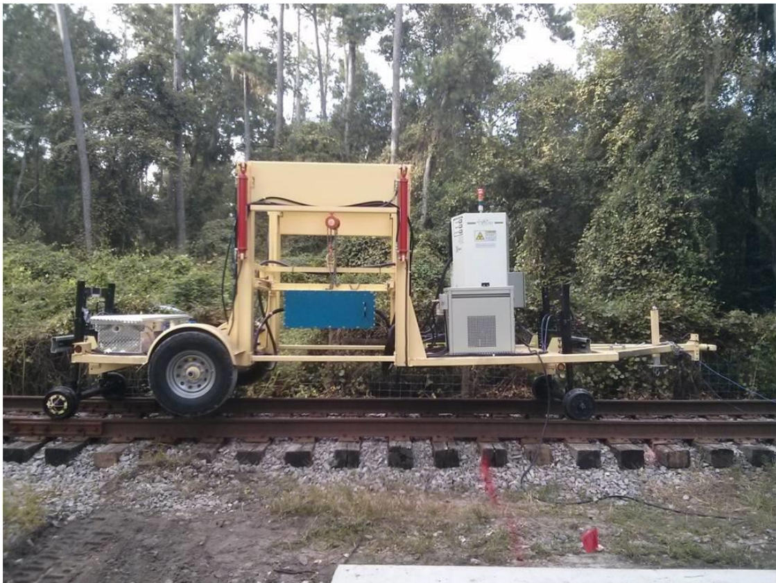
Figure 5: Research cart on the wood tie research track. The blue box in the center of the cart houses the Source.
