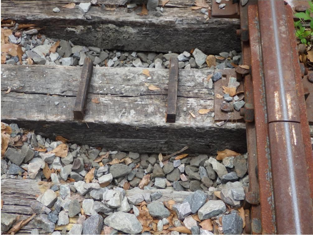
Figure 8: Tie surface before destructive examination. The void in the X-Ray image is between the two cross-member pieces of wood.
