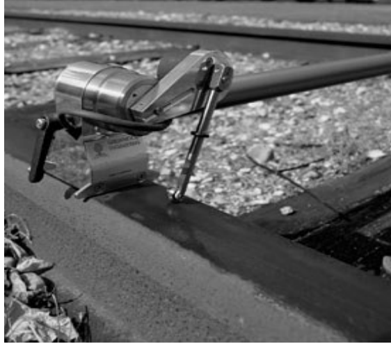
Figure 5.2: Rail profile measurement using MINIPROF rail profile system
